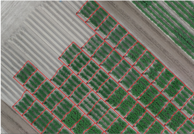
Figure 1.2: The figure shows the polygonal boundaries detected in the field of Kolumerwaard, in black is the plot number from the field scheme for seedlot association.
