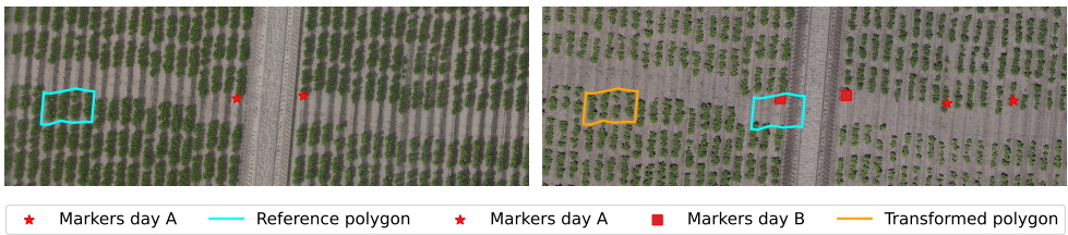
Figure 2.5: This figure illustrates the need for alignment. The markers and polygon found in day A (left panel) are not in the right spot in the coordinate system of day B (right panel), but using the day specific marker coordinates we can correctly transform day A's polygons to the coordinates of day B (orange polygon in the right panel) without needing to recompute them.
