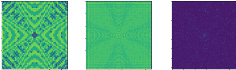
Figure 20: Comparison of converged solution quality for CoPILOT devices of different resolutions. The nearfield design case is considered, with hyperparameters N = 50 , S_f = 10.0 , L = 0.8 , and h_i = 0 . These plots show the electric field intensity produced on the focal plane by an optimized design. The first is produced by an optimized device with 50 \times 50 pixels, and at this resolution the scattering pattern typically reflects the blocky metasurface shape. The second comes from a device of resolution 100 \times 100 pixels, and this behaviour is somewhat reduced. The final device, at 150 \times 150 pixels, surpasses the \lambda/3 feature size limit at which metamaterial behavior emerges, and so is able to produce a much more favorable scattering pattern.
