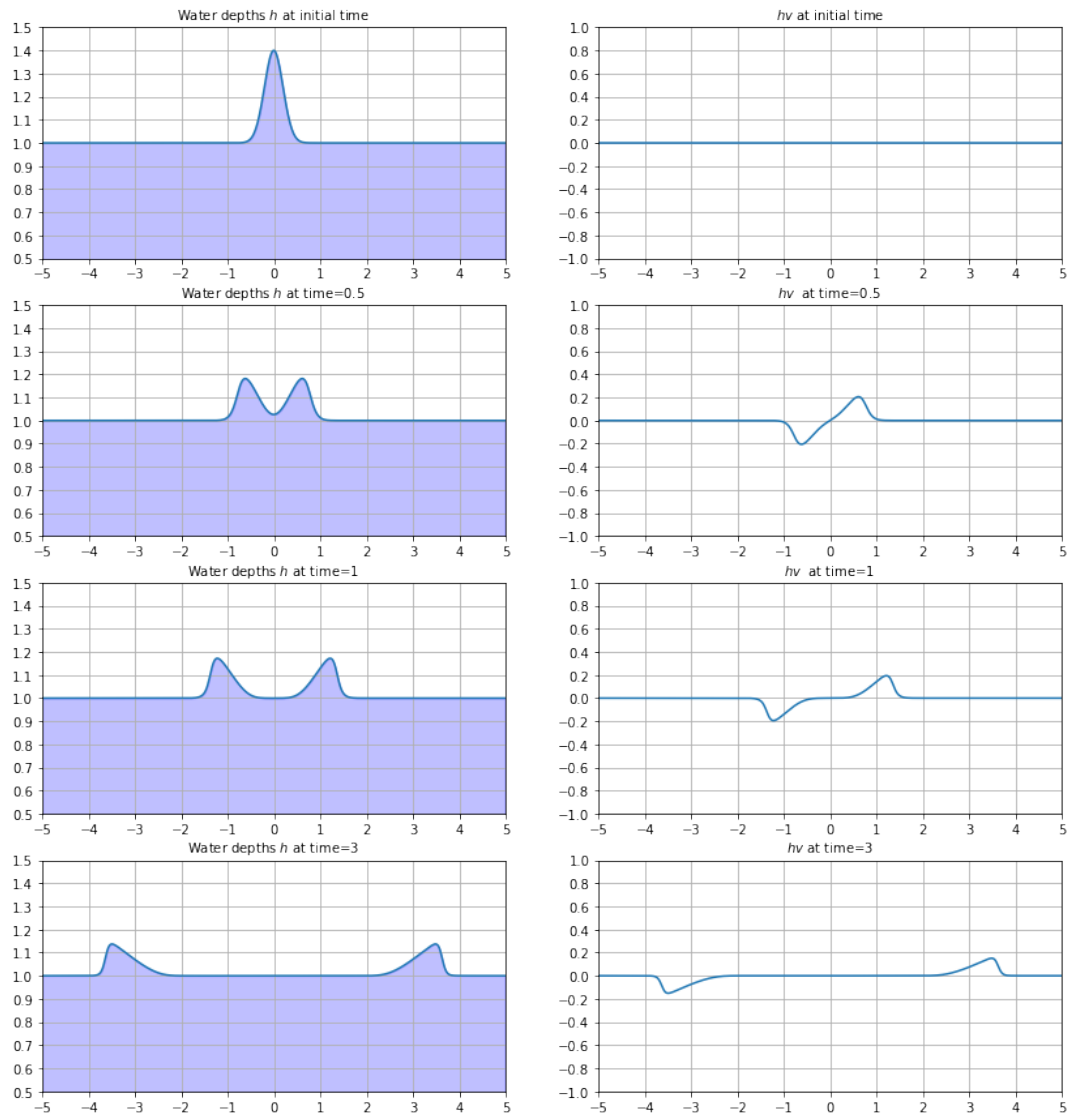
Figure 6.4: The results of the developed method for the shallow water equations for a hump of water with zero initial velocity and with zero source terms. The same initial data was considered as in [12] and the results turn out similar to those given on page 257 [12]. The figure on the left show the water depths and the figures on the right show the depths times the water velocities, which equals the discharges when the width is B = 1 .
