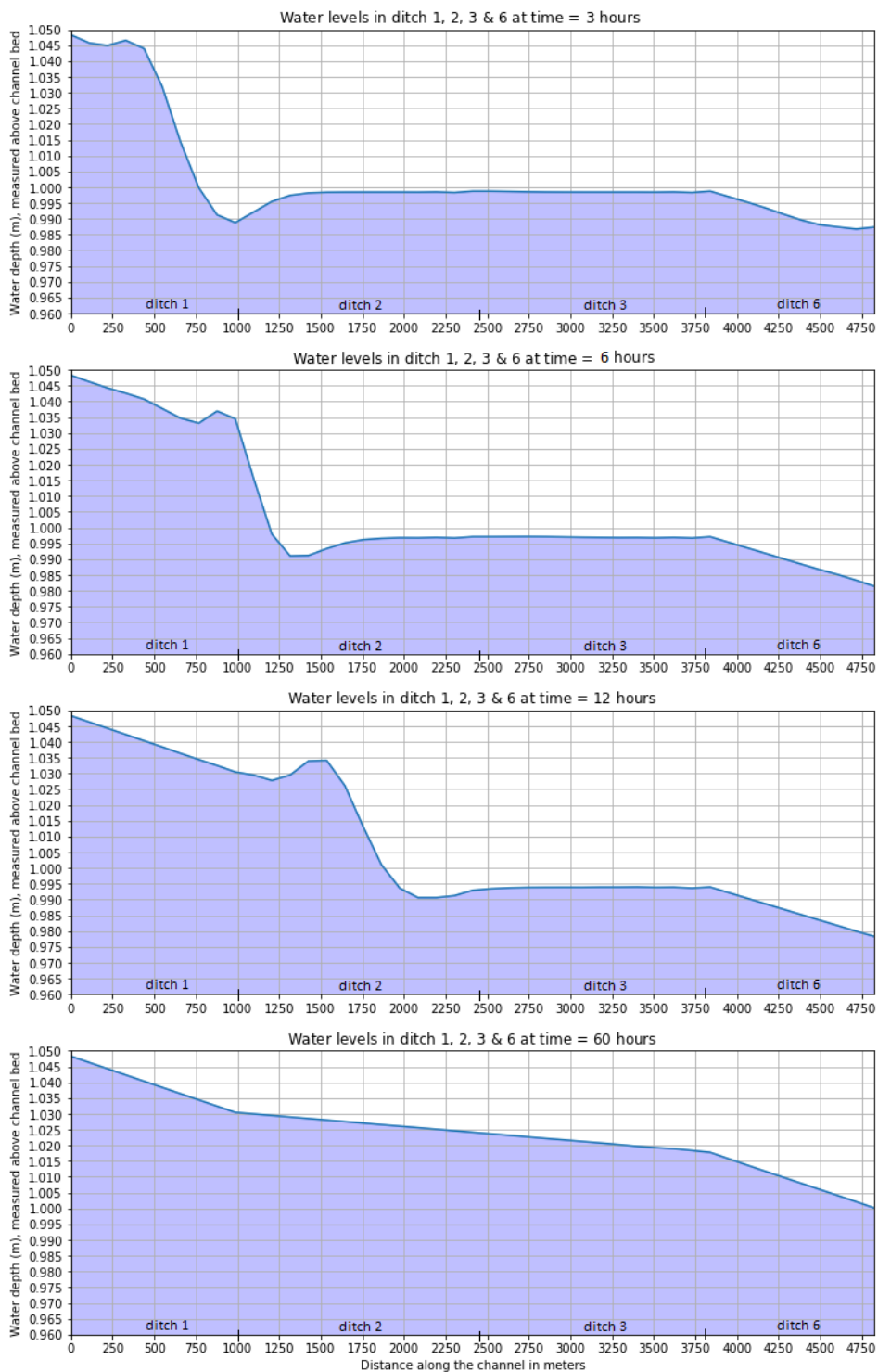
Figure 8.3: The results for water levels of the left branch of the network including ditches 1, 2, 3 and 6.
