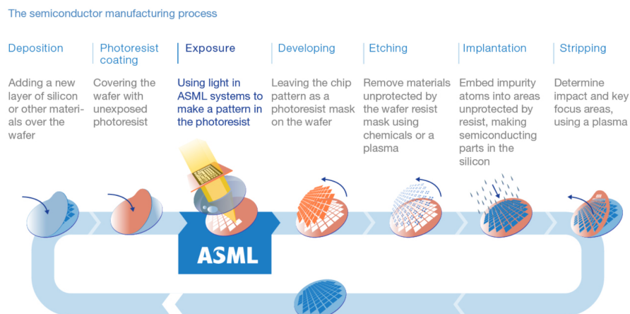
Figure 1.1: A summary of the semiconductor manufacturing process, taken from [1]. ASML develops the TwinScan machines that perform the exposure step.
