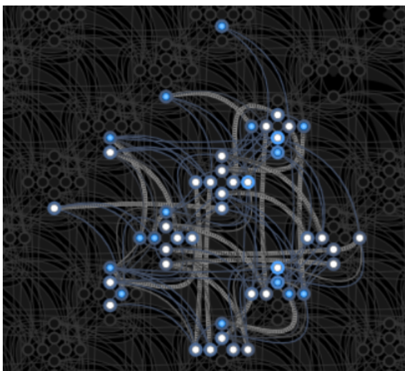
Figure 4.7: MOT instance of 27 variables embedded onto 49 qubits in Pegasus topology. Chains are in light gray. Measurement of one sample of the system is displayed on the qubits with circle filling blue corresponding to +1 and white to -1.
