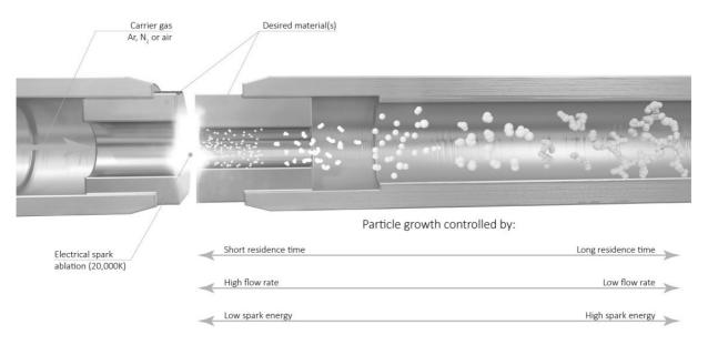
Next, the aerosol is transferred through a tube allowing the particles to grow due to coagulation and agglomeration. Particle growth is dependent on the material, flow rate, tube length, and spark energy, but other parameters may also be of influence.
