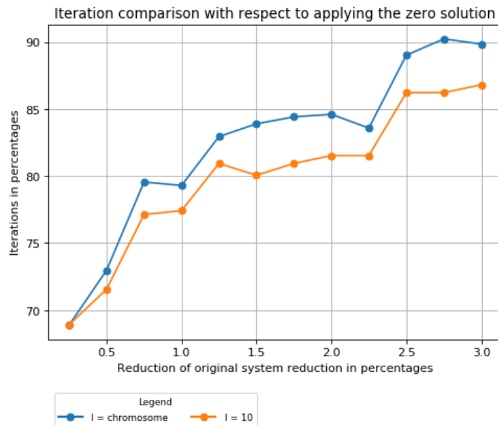
Figure 8.12: The amount of iterations needed for convergence by choosing the initial solution as the solution of the reduced original system.
