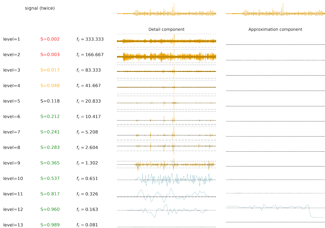
Figure H.7: Discrete wavelet filter to filter transient for signal presented in Figure 5.7a. (Discrete Wavelet Decomposition using the Symmlets 8 wavelet, upto level 9)
