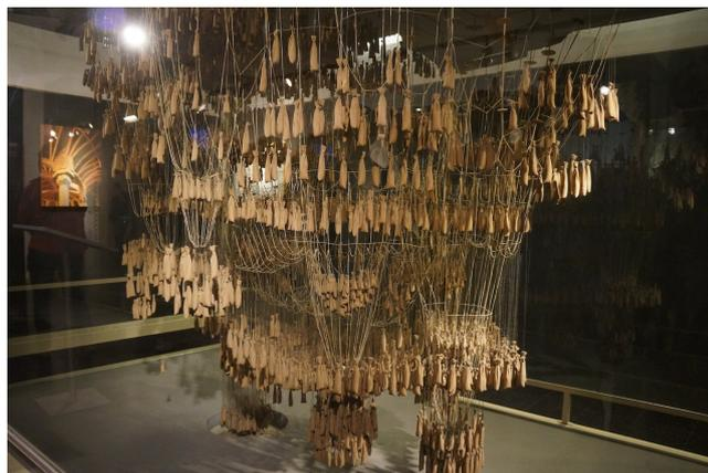
Figure 1.1: A replica of Gaudi's rope and sandbag model from La Sagrada Familia [22].
