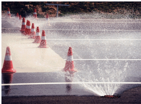
Figure 1.4: sprinkling the track for a hydroplaning test.
