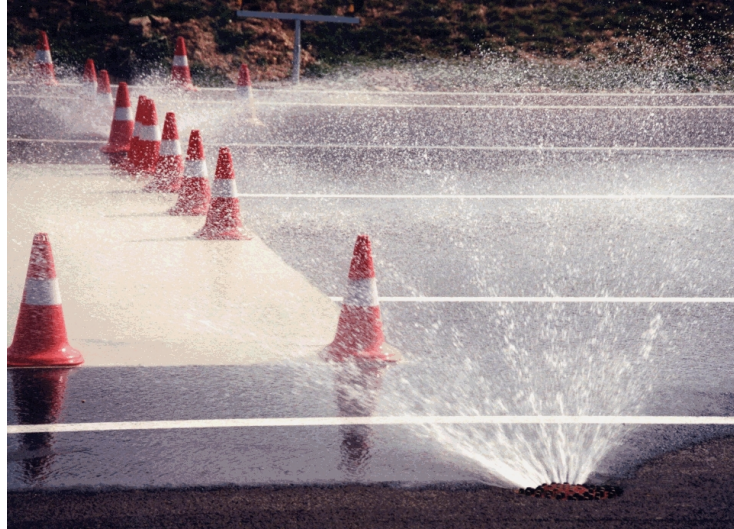
Figure 1.4: sprinkling the track for a hydroplaning test.
