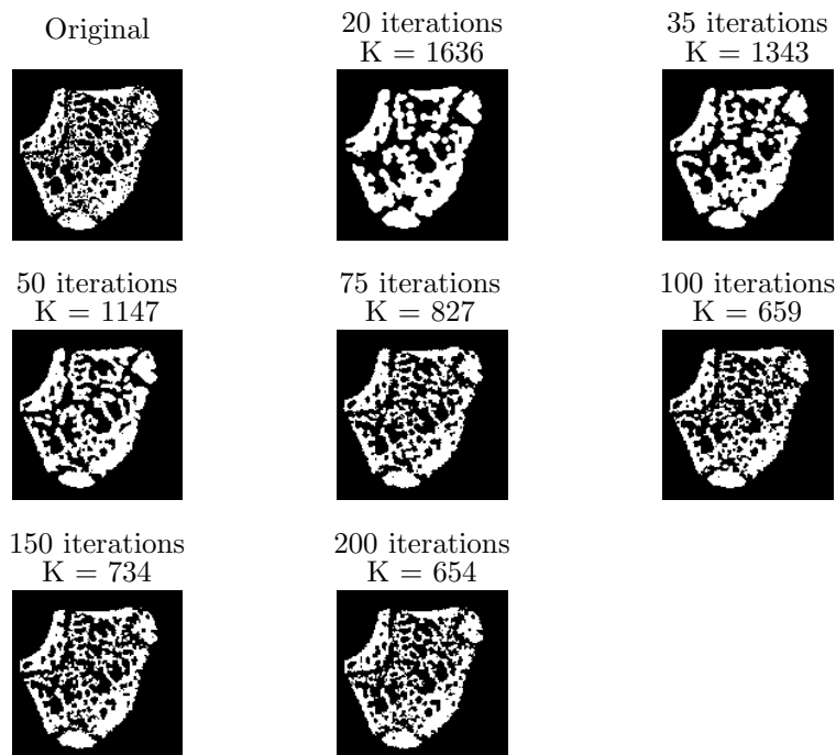
Figure 6.13: The performance of the new DART with the neighbours construct and SIRT as ARM for a various number of intermediate iterations. The test problem Phantom was scanned using 90 angles and the measurement data were polluted with 10^3 noise.
