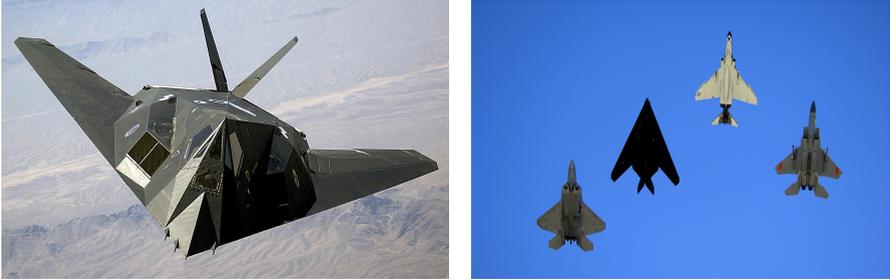
(a) The faceted shape of the airframe reduces the monostatic radar visibility.
