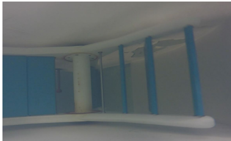
Figure 2.2: Snapshots reproduced from the testing of the OWM depicting the lamellas at the fully-open condition aligned with the flow
