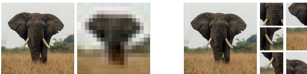
Figure 3.2: Visualization of downsampling/resizing (left) and patch cropping (right) for an example image.
