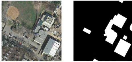
Figure 7.10: Image used to generate the feature maps for the Inria Aerial Image Dataset ( 512 \times 512 pixels, corresponding to 4 \times 4 subdomains). The corresponding mask is also shown on the right.
