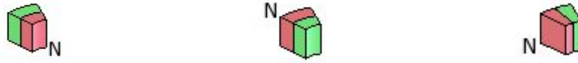
(a) Magnetised South on outside face, strength of 0.624 T on the outside radius. (b) Magnetised North on outside face, strength of 0.624 T on the outside radius. (c) Magnetised through circumference, strength of 0.721 T on the outside radius.
