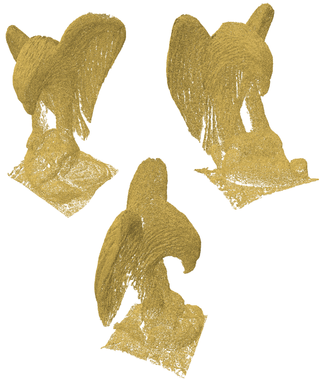
Figure 3. Different views of an eagle point cloud (from Open3D's datasets [18]). The point cloud (796,825 points) contains intricate features, making it an excellent candidate for evaluating reconstruction algorithms.
