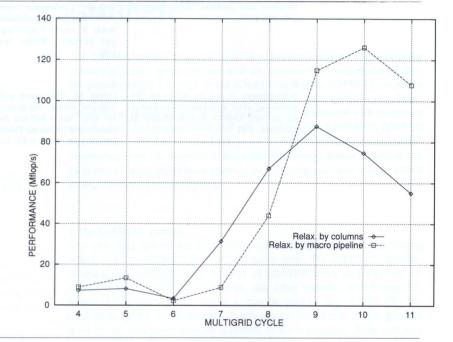
Figure 5. Performance on 16 cells of the parallel relaxation on the various grid levels (up to grid level 10), unoptimized version versus optimized version by macro pipelining.
