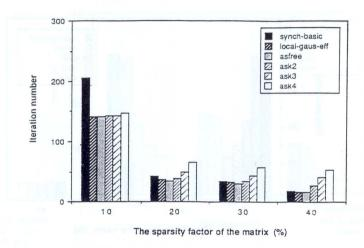
Figure 1. Number of iterations for matrices of size 3267 (sparse matrix type).
