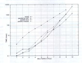
Figure 2. Comparison of the computing time for whole multigrid cycles between the serial case, the automatic parallelization by KAP, the parallelization along columns on four cells with four threads (slice) and sixteen threads (modular).
