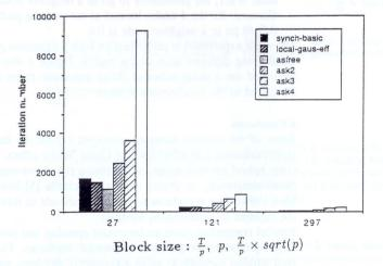
Figure 5. Number of iterations for matrices of size 3267 (tridiagonal matrix type).
