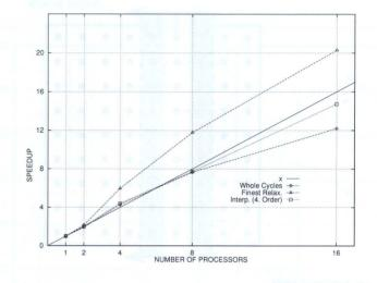
Figure 3. Speedup of the parallelization along columns on a various number of processors for all cycles up to level 10, and for the 4<sup>th</sup> order interpolation and the relaxation on level 10.
