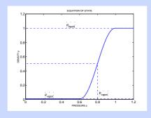
The pure liquid and pure vapor phase are nearly incompressible, while the mixture phase is highly compressible. As a result the Mach number in the flow varies in the range  $0 \le \mathrm{Ma} \le 30$ . This calls for a Mach uniform method: A method that has accuracy and efficiency nearly uniform in the Mach number[1]. A staggered discretisation in combination with a compressible pressure correction solution method has this desirable property.
