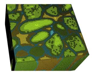
Figure: from CT scan to mesh, approx. 3 mln DOF
