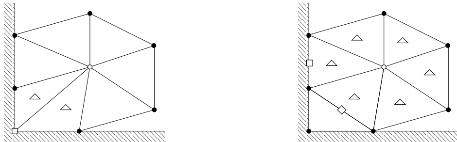
Figure 2: Boundary treatment: nodal vs. edgewise recovery.
